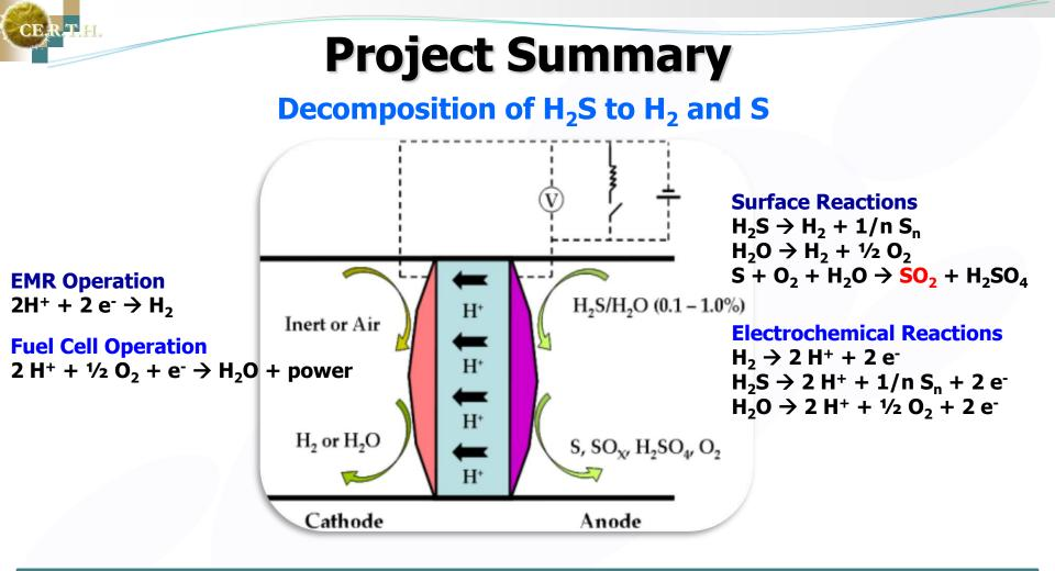
Anode is exposed to concentrated  $H_2S/H_2O$  mixtures (0.1-1%  $H_2S$ ) and catalyzes the decomposition of  $H_2S$  to  $H^+$  and S.
